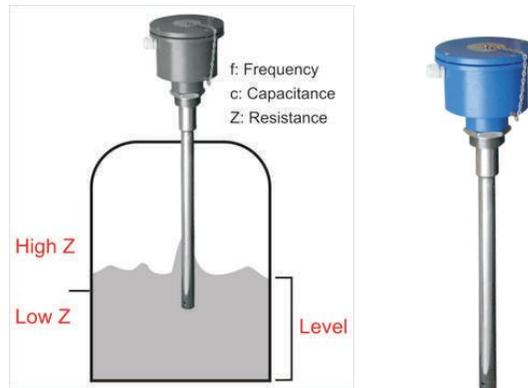
Head mounted electronics converts the capacitance variation to 4-20mA signal for long distance transmission. It is provided with trimpots for SPAN and ZERO adjustments. With no moving parts it is free from wear and tear, rugged and robust in construction. No dead zone like float based instruments.
